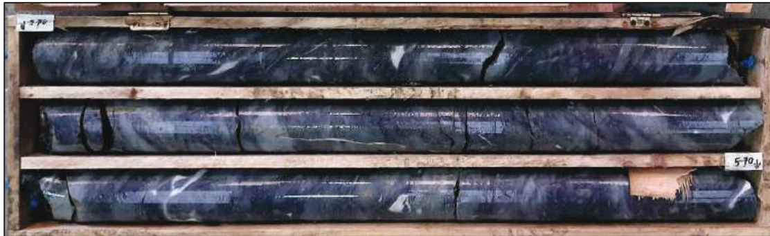
Photo 1 – Core recovery at RC01 (2.7 to 5.7 m)
