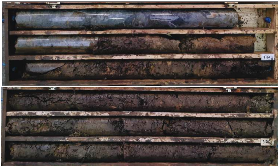
Photo 2 – Core recovery at RC02 (3.6 to 9.6 m)
